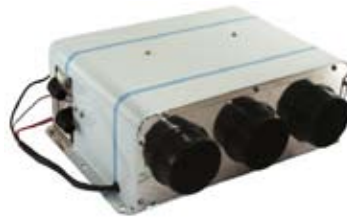
060216 Cabin Heater 12 V., 60 Watt - Speed 1, 77 Watt - Speed 2, 114 Watt - Speed 3, Airflow-Speed 1 264 m³/h, Water connection 16 mm, Regulation Yes Blower: Cargo 160483.
