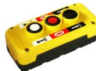
181245 Control Box 220 V. - AC, 24 V. - DC, 5 Amp.-Max, Buttons 3, Protection degree IP 65 Lift-stop-lower operated by spring return push button.
