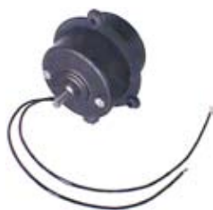
060060 Cabin Heater Motor Servicing: Cargo 060057. 24 V., 24 Watt, Length 63 mm, Shaft dimension 6.35 x 16 mm, Diameter 70 mm
