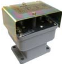
180290 Battery Switch Relay For serial and parallel connection of two 12V. batteries in 12V. systems w/ 24V. starter.
