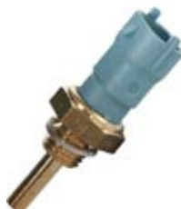
181395 7.3239 Engine Management Temp. Transmitter Servicing: Alfa Romeo, Citroen, Fiat, Iveco, Lancia, Opel, Peugeot, Saab Thread M12 - 1.5 Replacing original light blue, white and black sensor.
