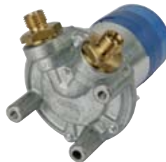
070019 Fuel Pump Servicing: Bobcat. 12 V., Capacity 120 L/h, Fuel Petrol, Pressure (bar) 0.1 Thread R-1/4". Suction 0.2 bar = 2.7 mtr.
