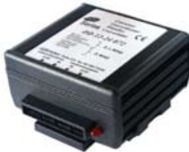
160642 Converter 12 V. In, 24 V. Out, 4 Amp. (5 min), 3 Amp.-Cont, 72 Watt - Out, Dimension 89 x 87 x 50
