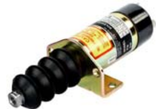
090224 Shutdown Solenoid 12 V., 17 Amp. pull , 0.25 Amp. hold , Thread 6, Return spring 17N, Pull rating 40N at 25.4 mm, Hold rating 89N
