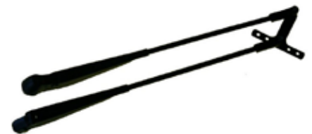
160339 Wiper Arm Length 400 mm, Wiper arms distance 57 mm, Mount. on wiper shaft dimension Ø: 6 mm + M8 shaft, Adjustable length No Usable w/ wiper motor: Cargo 160292 and 106293.
