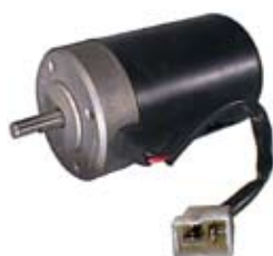
160005 Universal Motor 12 V., 40 Watt, Length 121 mm, Shaft dimension 8 x 22 mm, Diameter 60 mm, Speed 1 - speed, Revolutions 2000 Universal.
