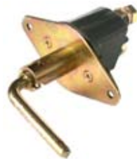
180211 Battery Main Switch 24 V., 2500 Amp. (5 min), 250 Amp.-Cont, Type Battery, No. of mounting holes 2, Mounting holes distance 100 mm, Material Metal, Key Yes, Protection degree IP 65 Spare key: Cargo 180288 or 180333. Rubber boot: Cargo 180375.
