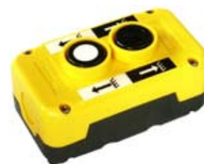
181244 Control Box 220 V. - AC, 24 V. - DC, 5 Amp.-Max, Buttons 2, Protection degree IP 65 Lift and lower operated by spring return push button.
