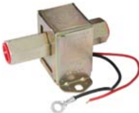
070201 Fuel Pump 12 V., Capacity 113 L/h, Fuel Diesel, Pressure (Kg) 0.31 - 0.62, Pressure (Psi) 4.5 - 9, Pressure (bar) 0.3 - 0.6 Suitable w/ canola oil. Hose connection 3/8-18.
