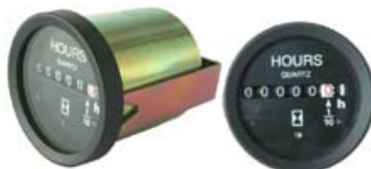
160702 Hour Meter 12 - 28 V., Colour Black, O.D. 52 mm, Mounting Hook fastening w/o illumination.
