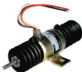
090199 Shutdown Solenoid 12 V., 46 Amp. pull, 1.1 Amp. hold, Thread 6, Return spring 17N, Pull rating 89N ved 25.4 mm, Hold rating 178N Syncro start / Woodward. Red=Hold, White=Pull, Black=Ground.
