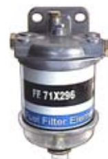
090194 Filter Assy Thread 1/2"-20 UNF, Hand pump No, Water separator Yes Flow 150 L/h.
