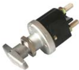
180289 Battery Main Switch 24 V., 2500 Amp. (5 min), 250 Amp.-Cont, Type Battery, No. of mounting holes 2, Mounting holes distance 38 mm, Material Metal, Key Yes, Protection degree IP 65 Rubber boot: Cargo 180375.
