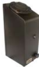
060222 Cabin Heater 12 V., Airflow-Speed 1 76 m³/h, Water connection 12 mm, Regulation No Heat-on 1331-12.
