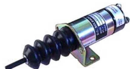
090110 Shutdown Solenoid 24 V., 17 Amp. pull, 0.25 Amp. hold, Thread 6, Return spring 9N, Pull rating 40N at 25.4 mm, Hold rating 89N Syncro start / Woodward.
