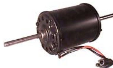
160252 Universal Motor 24 V., Length 102 mm, Shaft dimension 80 x 65 mm, Diameter 82 mm, Speed 1 - speed Universal.
