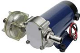
070209 Electrical Fluid Pump HD 24 V., Capacity 40 L/min, Dimension 212 x 174 x 109, Hose connection 16 mm, Pressure (Psi) 36, Pressure (bar) 2.5 Model UP12. Self priming 4 m.
