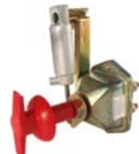
180279 Battery Main Switch 24 V., 2500 Amp. (5 min), 250 Amp.-Cont, Type Battery, No. of mounting holes 2, Mounting holes distance 110 mm, Material Plastic, Poles 1, Key Yes, Explosionproof Yes, Pneumatic Yes, Protection degree IP 65 Rubber boot: Cargo 180375. Spare key: Cargo 180292.
