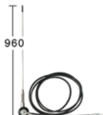
040177 Aerial Length 950 mm, Hole size 8 mm, Mounting angle 0 - 90°, Cable length 2.1 m, Material Stainless steel Extended. 2 sections.
