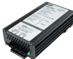
160960 Power Converter Servicing: Used for mounting computers in trolleys. 10 - 32 V. In, 12 V. Out, 6 Amp.-Cont, 72 Watt - Out, Dimension 167 x 87 x 50, Protection degree IP533 Modified to stabilize the output voltage.
