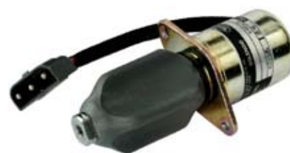
090226 Shutdown Solenoid 24 V., 24 Timermodul V., 25 Amp. pull, 0.5 Amp. hold, Thread 6, Return spring 7N, Pull rating 111N at 25.4 mm, Hold rating 182N Syncro start / Woodward. Red=Common. White=Pull. Yellow=Hold.
