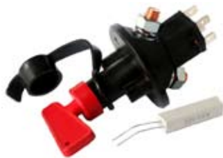
180596 Battery Main Switch 12 V., 500 Amp. (5 min), 100 Amp.-Cont, Type Battery, No. of mounting holes 2, Mounting holes distance 38 mm, Material Plastic, Secondary circuit Yes, Key Yes Spare key: Cargo 180029.
