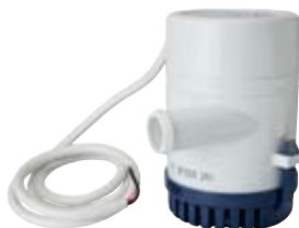
070185 Bilge Pump 24 V., Capacity 95 L/min, Type Bilge, Lift height 4 m, Dimension 160 x 96, Hose connection 26.5 mm Model UP1500.
