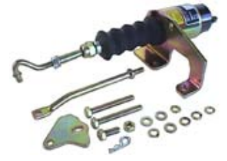
090097 Solenoid Shutdown Kit 1.1 Amp., Pull rating 89N at 25.4 mm, Hold rating 178N Syncro start / Woodward. Internal.
