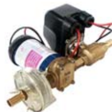
070172 Water Pump 24 V., Capacity 14 L/min, Type Water, Dimension 163 x 249 x 118, Hose connection 14 mm, Pressure (Psi) 29, Pressure (bar) 2 Model UP4A. Self priming 1.5 m.
