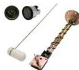
160872 Fuel Gauge 24 V., Type Electrical operated, Colour Black, O.D. 52 mm, Mounting Hook fastening
