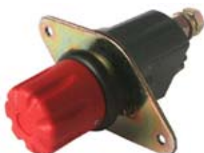
180326 Battery Main Switch 24 V., 2500 Amp. (5 min), 250 Amp.-Cont, Type Battery, No. of mounting holes 2, Mounting holes distance 100 mm, Protection degree IP 65 Rubber boot: Cargo 180375.
