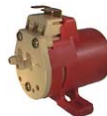
160223 Washer Pump Servicing: Peugeot 104, 504. 12 V., Capacity 1500 ml/min, Type Single For independent mounting in engine compartment.
