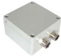
160167 Relay Box Servicing: For 12V. trailer pulled by a 24V. vehicle. 12 / 24 V., 10 Amp., 250 Watt, No. of poles 7 Switches the voltage from 24V to 12V by 5 relays. Run at 24V and leading 12V from one of the batteries or converter to the lamps of the trailer. For continuous use it has to be connected via a converter. For internal mounting.
