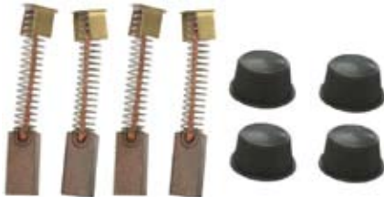
070182 Brush Set Servicing: Cargo 070144, -145, -149, -150, -152. Height 8.6 mm, Length 18.1 mm, Thickness 5.6 mm
