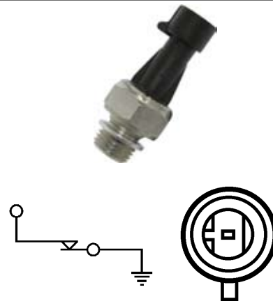
180689 7.0096 Oil Pressure Switch Servicing: Alfa Romeo, Citroen, Fiat, Innocenti, Iveco, Lancia, Opel, Peugeot, Suzuki Thread M14 - 1.5, Pressure 0.3 bar
