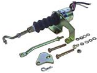
090099 Solenoid Shutdown Kit 0.5 Amp., Pull rating 89N at 25.4 mm, Hold rating 178N Syncro start / Woodward. External.
