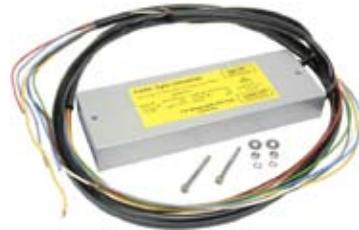
160901 Trailer Light Converter 24 V. In, 12 V. Out Output: 2 x 42W + 4 x 60W. Level B. To be used when Cargo 160899 and 160900 are not suited.
