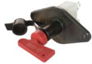
180229 Battery Main Switch 24 V., 2500 Amp. (5 min), 250 Amp.-Cont, Type Battery, No. of mounting holes 2, Mounting holes distance 100 mm, Material Plastic, Key Yes, Protection degree IP 66 Spare key: Cargo 180029.
