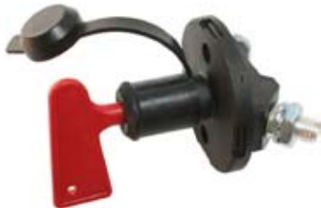
180028 Battery Main Switch 24 V., 500 Amp. (5 min), 100 Amp.-Cont, Type Battery, No. of mounting holes 2, Mounting holes distance 38 mm, Material Plastic, Key Yes Spare key: Cargo 180029 or 180143. Pole: Ø 10 mm.
