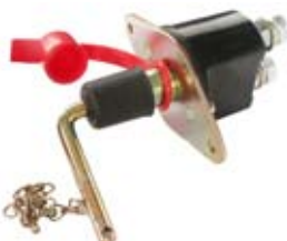
181238 Battery Main Switch 24 V., 2500 Amp. (5 min), 250 Amp.-Cont, Type Battery, No. of mounting holes 2, Mounting holes distance 38 mm, Material Metal, Key Yes Rubber boot for terminals: Cargo 180375.
