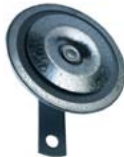
160393 Horn 36 - 48 V., 335 Hz, Type Single tone., E-approved Yes
