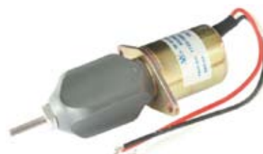
090348 Shutdown Solenoid 12 V., 46 Amp. pull, 1.1 Amp. hold, Thread 6, Return spring 4-8N, Pull rating 111N at 25.4 mm, Hold rating 182N Syncro start / Woodward.
