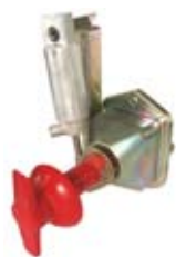
180291 Battery Main Switch 24 V., 2500 Amp. (5 min), 250 Amp.-Cont, Type Battery, No. of mounting holes 2, Mounting holes distance 110 mm, Material Plastic, Poles 2, Key Yes, Explosionproof Yes, Pneumatic Yes, Protection degree IP 65
