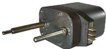
160292 Wiper Motor 12 V., Distance between shafts 57 mm, Wiper angle 110°, Wiper shaft w/ 2 shafts for parallelogram
