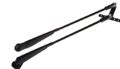
160257 Wiper Arm Length 400 mm, Wiper arms distance 57 mm, Mount. on wiper shaft dimension M6 cone + M8 shaft, Adjustable length No Usable w/ wiper motor: Cargo 160258, 160290, 160291, 160357, 160408.
