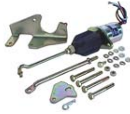
090106 Solenoid Shutdown Kit Servicing: Nippodenso, Zexel. 0.63 Amp., Pull rating 89N at 25.4 mm, Hold rating 178N Syncro start / Woodward. External.
