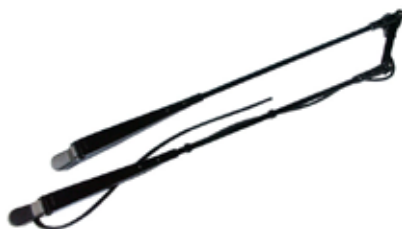
160608 Wiper Arm Length 680 mm, Wiper arms distance 110 mm, Mount. on wiper shaft dimension 2 x M8 cone
