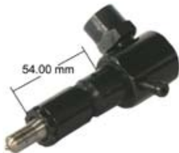
100598 Injector Servicing: Yanmar air cooled single cylinder. Engine Type: YDLL. YPFE-M. Fitted w/ nozzle DLLA150p224 opening pressure: 196 bar.
