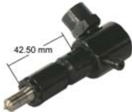
100597 Injector Servicing: Yanmar air cooled single cylinder. Engine Type: YDLL. YPFE-M. Fitted w/ nozzle DLLA150p224 opening pressure: 196 bar.
