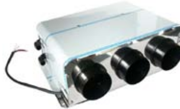
060220 Cabin Heater 24 V., 60 Watt - Speed 1, 77 Watt - Speed 2, 114 Watt - Speed 3, Airflow-Speed 1 264 m³/h, Water connection 16 mm, Regulation No Blower: Cargo 160649.
