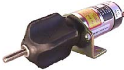
090160 Shutdown Solenoid Servicing: Universal. 12 V., 30 Amp. pull , 0.7 Amp. hold , Thread 6, Return spring 17N, Pull rating 40N at 25.4 mm, Hold rating 89N Syncro start / Woodward.
