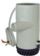
070157 Bilge Pump 12 V., Capacity 126 L/min, Type Bilge, Lift height 4 m, Dimension 200 x 96, Hose connection 31.8 mm Model UP2000.
