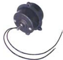
060059 Cabin Heater Motor Servicing: Cargo 060056. 12 V., 24 Watt, Length 63 mm, Shaft dimension 6.35 x 16 mm, Diameter 70 mm Heat-on.
