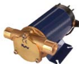
070145 Water Pump 24 V., Capacity 35 L/min, Dimension 176 x 120 x 94, Hose connection 25 mm, Pressure (Psi) 11.6, Pressure (bar) 0.8 Model UP1-N. Self priming 1.5 m.
