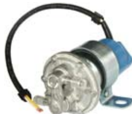
070184 Fuel Pump Servicing: VW marine. 12 V., Capacity 120 L/h, Fuel Benzin, diesel, ethanol, methanol, Pressure (bar) 0.1 8 mm hose connection. Waterproof. Suction 0.2 Bar = 2.7 mtr.
