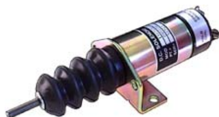
090109 Shutdown Solenoid Servicing: Universal. 12 V., 30 Amp. pull, 0.7 Amp. hold, Thread 6, Return spring 9N, Pull rating 40N at 25.4 mm, Hold rating 89N Syncro start / Woodward.
