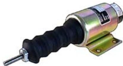
090168 Shutdown Solenoid Servicing: Universal. 12 V., 44 Amp. pull , 0.6 Amp. hold , Thread 6, Return spring 35N, Pull rating 75N at 25.4 mm, Hold rating 178N Syncro start / Woodward.
