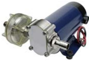
070208 Electrical Fluid Pump HD 12 V., Capacity 40 L/min, Hose connection 16 mm, Pressure (Psi) 36, Pressure (bar) 2.5 Model UP12. Self priming 4 m.
