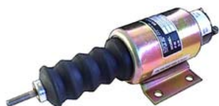
090111 Shutdown Solenoid 12 V., 44 Amp. pull, 0.6 Amp. hold, Thread 1/4", Return spring 35N, Pull rating 75N at 25.4 mm, Hold rating 178N Syncro start / Woodward.
