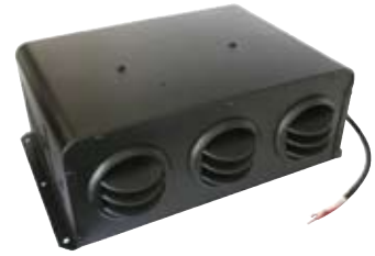
060234 Cabin Heater 12 V., Airflow-Speed 1 264 m³/h, Water connection 16 mm, Regulation Yes
