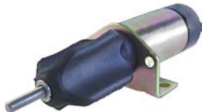
090161 Shutdown Solenoid Servicing: Universal. 24 V., 17 Amp. pull , 0.25 Amp. hold , Thread 6, Return spring 17N, Pull rating 40N at 25.4 mm, Hold rating 89N Syncro start / Woodward.
