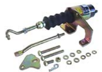
090101 Solenoid Shutdown Kit 0.5 Amp., Pull rating 89N at 25.4 mm, Hold rating 178N Syncro start / Woodward. Internal.
