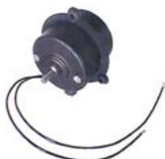
060214 Cabin Heater Motor Servicing: Cargo 060211. 24 V., 50 Watt, Length 63 mm, Shaft dimension 6.35 x 16 mm, Diameter 70 mm, Speed 1 - speed
