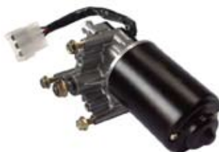
160408 Wiper Motor 24 V., Distance between shafts 57 mm, Wiper angle 95°, Wiper shaft w/ 2 shafts for parallelogram
