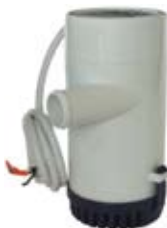
070186 Bilge Pump 24 V., Capacity 126 L/min, Lift height 4 m, Dimension 200 x 96, Hose connection 31.8 mm Model UP2000.
