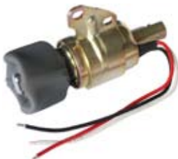
090371 Shutdown Solenoid Servicing: Kubota D722, Z482. 24 V., 25 Amp. pull , 0.5 Amp. hold
