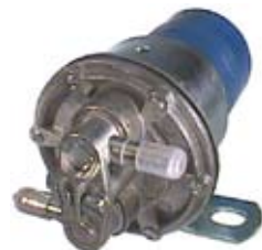
070021 Fuel Pump Servicing: VW 12 V., Capacity 120 L/h, Pressure (bar) 0.1 Hose nipple 8 mm. Suction 0.2 bar = 2.7 mtr. Gasoline/diesel. Connectors can be rotated.
