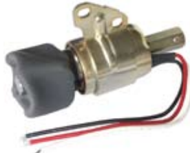
090370 Shutdown Solenoid Servicing: Kubota D722, Z482. 12 V., 46 Amp. pull , 1.1 Amp. hold
