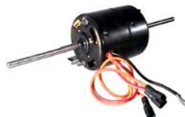
160250 Universal Motor 12 V., Length 105 mm, Shaft dimension 10 x 110 mm, Diameter 90 mm, Speed 3 - speed Universal.
