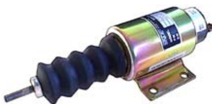
090113 Shutdown Solenoid 24 V., 23 Amp. pull, 0.3 Amp. hold, Thread 6, Return spring 35N, Pull rating 75N at 25.4 mm, Hold rating 178N Syncro start / Woodward.
