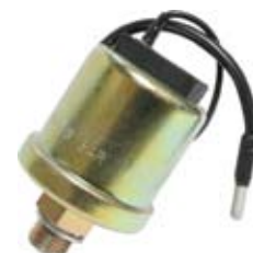
180702 7.0602 Oil Pressure Sensor Servicing: Fiat, Innocenti, Lancia, Seat Thread M14 - 1.5, Working area 0-8
