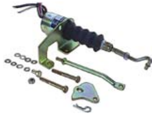
090096 Solenoid Shutdown Kit 1.1 Amp., Pull rating 89N at 25.4 mm, Hold rating 178N Syncro start / Woodward. External.
