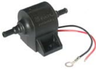
070191 Fuel Pump 12 V., Capacity 151 L/h, Fuel Benzin, diesel, ethanol, methanol, Pressure (Kg) 0.5 - 0.7, Pressure (Psi) 7 - 10 Standard 6 mm hose nipples.
