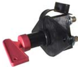
180203 Battery Main Switch 24 V., 2500 Amp. (5 min), 250 Amp.-Cont, Type Battery, No. of mounting holes 2, Mounting holes distance 100 mm, Material Plastic, Key Yes, Protection degree IP 66 Spare key: Cargo 180029.
