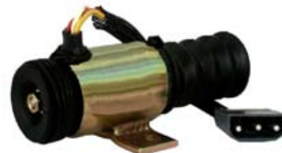
090281 Shutdown Solenoid Servicing: Volvo. 24 V., 25 Amp. pull, 0.5 Amp. hold, Thread 6, Pull rating 89N at 25.4 mm, Hold rating 236N Syncro start / Woodward.
