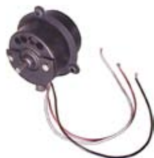
060213 Cabin Heater Motor Servicing: Cargo 060210. 12 V., 50 Watt, Length 63 mm, Shaft dimension 6.35 x 16 mm, Diameter 70 mm 2 speed.
