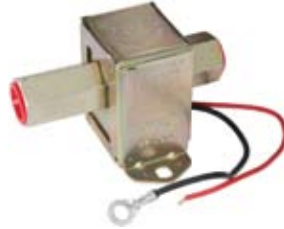
070202 Fuel Pump 24 V., Capacity 113 L/h, Fuel Diesel, Pressure (Kg) 0.31 - 0.62, Pressure (Psi) 4.5 - 9 Suitable w/ canola oil. Hose connection 3/8-18.
