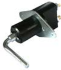
180087 Battery Main Switch 24 V., 2500 Amp. (5 min), 250 Amp.-Cont, Type Battery, No. of mounting holes 2, Mounting holes distance 100 mm, Material Metal, Key Yes Spare key: Cargo 180202.
