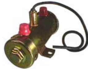
070004 Fuel Pump 24 V., Capacity 113.5 L/h, Pressure (Psi) 4 - 5 Incl. 2 pcs 6 mm hose nipples. 8 mm = Cargo 080955. 8 mm angle = Cargo 070181. 10 mm = Cargo 081154.
