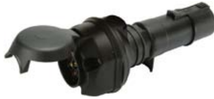
160900 Trailer Light Converter Adapter 24 V. In, 12 V. Out, 6 x 70 Watt - Out Max output 220W. 7 - 7 pole.
