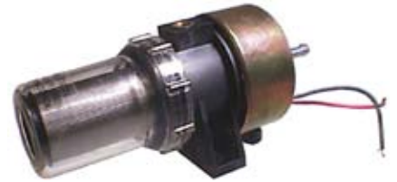
070076 Fuel Pump 12 V., Capacity 113 L/h, Fuel Benzin, diesel, ethanol, methanol, Pressure (Psi) 9- 11.5 w/ integral filter.
