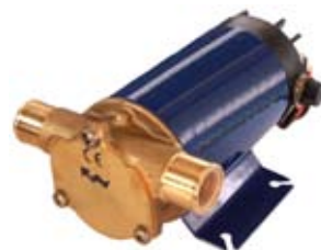
070144 Water Pump 12 V., Capacity 35 L/min, Dimension 176 x 120 x 94, Hose connection 25 mm, Pressure (Psi) 11.6, Pressure (bar) 0.8 Model UP1-N. Self priming 1.5 m.
