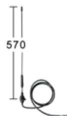
040190 Aerial Colour Black, Length 570 mm, Hole size 18 mm, Mounting angle 0 - 45°, Cable length 1.3 m, Material Fiber glass Removable mast.
