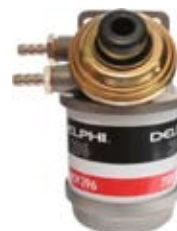
090203 Filter House Servicing: Ford Fiesta, Mondeo, Transit. Thread M14 - 1.5, Hand pump Yes, Water separator Yes 150 L/h.
