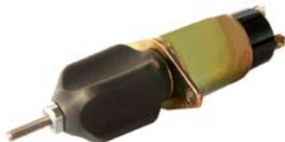
090297 Shutdown Solenoid 24 V., 46 Amp. pull, 1.1 Amp. hold, Thread 6, Return spring 7-11N, Pull rating 107N at 25.4 mm, Hold rating 169N
