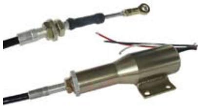
090368 Shutdown Solenoid 12 V., 12 Timermodul V. , 61 Amp. pull , 0.86 Amp. hold , Pull rating 129N at 25.4 mm, Hold rating 182N Syncro start / Woodward.
