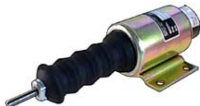
090169 Shutdown Solenoid Servicing: Universal. 24 V., 23 Amp. pull , 0.3 Amp. hold , Thread 6, Return spring 35N, Pull rating 75N at 25.4 mm, Hold rating 178N Syncro start / Woodward.
