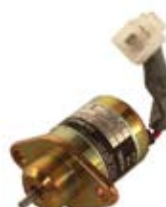
090216 Shutdown Solenoid Servicing: Kubota. 12 V., 30 Amp. pull, 0.7 Amp. hold, Type Stop solenoid, Return spring 17N, Pull rating 44 N at 25.4 mm, Hold rating 85N
