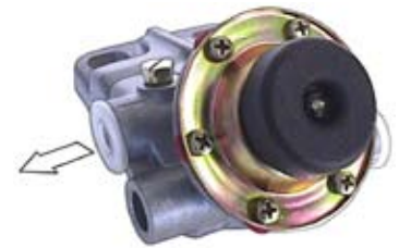
090166 Filter Cover Thread M14 - 1.5, Hand pump Yes Filter thread 16 x 1.5 mm.
