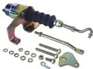
090102 Solenoid Shutdown Kit 0.5 Amp., Pull rating 89N at 25.4 mm, Hold rating 178N Syncro start / Woodward. Internal.
