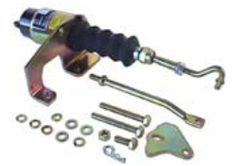
090098 Solenoid Shutdown Kit 1.1 Amp., Pull rating 89N at 25.4 mm, Hold rating 178N Syncro start / Woodward. Internal.
