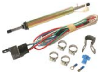
081176 Fuel Heater 12 V., 150 Watt, Type Electric, Demister tube connection 8/10 mm, Sandwich tipe No
