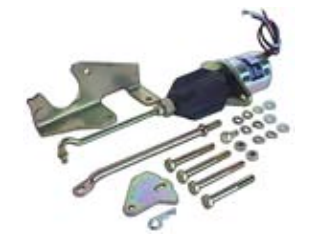
090103 Solenoid Shutdown Kit Servicing: Nippodenso, Zexel. 1.1 Amp., Pull rating 89N at 25.4 mm, Hold rating 178N Syncro start / Woodward. External.
