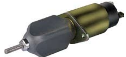
090210 Shutdown Solenoid 12 V., 46 Amp. pull , 1.1 Amp. hold , Thread 1/4 - 28, Return spring 9N, Pull rating 89N at 25.4 mm, Hold rating 178N
