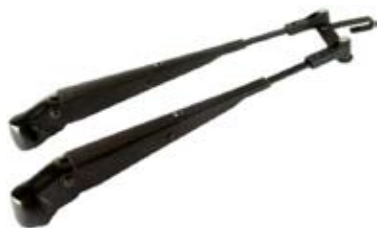
160484 Wiper Arm Length 340 - 420 mm, Wiper arms distance 57 mm, Mount. on wiper shaft dimension M8 cone + M8 shaft, Adjustable length Yes
