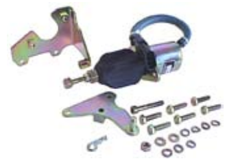
090108 Solenoid Shutdown Kit 0.63 Amp., Pull rating 89N at 25.4 mm, Hold rating 178N Syncro start / Woodward. External.
