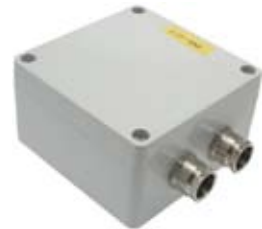
160797 Relay Box 12 - 12 V., 5 x 8 Amp., 5 x 250 Watt To reduce voltage drop, if you use vehicles w/ trailer. Fitted w/ 5 x 12V relays the 12V function will not be affected.
