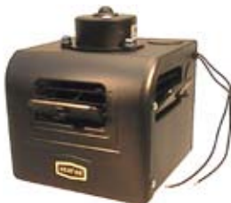
060211 Cabin Heater 24 V., Airflow-Speed 1 360 m³/h, Water connection 16 mm
