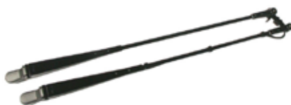
160571 Wiper Arm Length 680 mm, Wiper arms distance 60 mm, Mount. on wiper shaft dimension 2 x M8 cone
