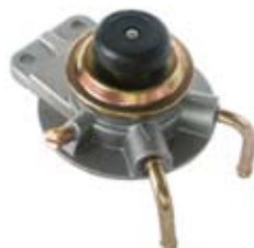
090347 Filter Top Servicing: Japanese appl. Thread 20 x 1.5, Hand pump Yes, Universal Yes 8 mm hose I.D.
