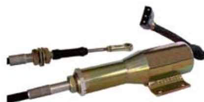
090267 Shutdown Solenoid Servicing: Volvo Wheel loader. 24 V., 39 Amp. pull, 0.86 Amp. hold, Pull rating 129N at 25.4 mm, Hold rating 182N Syncro start / Woodward.
