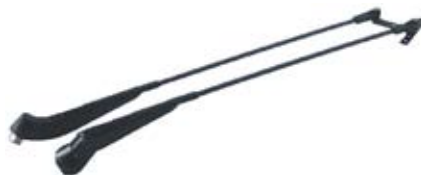
160256 Wiper Arm Length 450 mm, Wiper arms distance 57, Mount. on wiper shaft dimension M6 cone + M8 shaft, Adjustable length No Usable w/ wiper motor: Cargo 160258, 160290, 160291, 160357, 160408.
