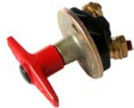
180271 Battery Main Switch 12/24 V., 1000 Amp. (5 min), 300 Amp.-Cont, Type Battery, No. of mounting holes 2, Mounting holes distance 45 mm, Material Plastic, Poles 10, Key Yes, Waterproof Yes, Protection degree IP 65 Rubber boot: Cargo 180375. Working temp. -30C°/+65C°.
