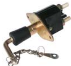
181475 Battery Main Switch 24 V., 2500 Amp. (5 min), 250 Amp.-Cont, No. of mounting holes 2, Mounting holes distance 100 mm, Protection degree IP 65 Spare key: Cargo 180288, w/o chain and rubber cap. Rubber boot: Cargo 180375
