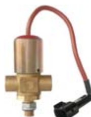
081046 Electro Valve 12 V., 12 Timermodul V., Thread M14 - 1.5 Can be used as emergency stop. 3-way. Electro valve.
