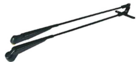
160358 Wiper Arm Length 500 mm, Wiper arms distance 57 mm, Mount. on wiper shaft dimension M6 cone + M8 shaft, Adjustable length No Usable w/ wiper motor: Cargo 160258, 160290, 160291, 160357, 160408.
