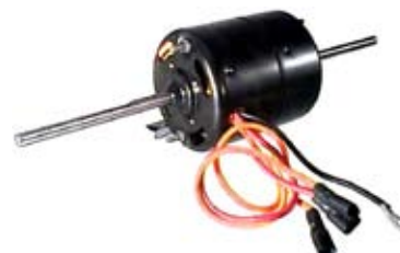
160251 Universal Motor 24 V., Length 107 mm, Shaft dimension 10 x 110 mm, Diameter 90 mm, Speed 3 - speed Universal.
