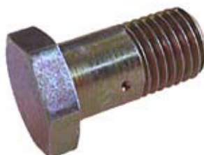
080114 Hollow Screw Hole size 0.55 cm, Thread M12 - 1.5
