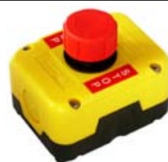
181247 Emergency Stop Button Protection degree IP65 Emergency stop button operable w/ push button, turn for reset.
