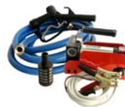
070162 Diesel Transfer/Filter Kit 12 V., Capacity 40 L/min, Type Fluid, Pressure (bar) 1.1 Tank kit 12V incl 2.5 m suction hose. 2.5 m pressure hose w/ gun, wire connection w/ alligator clips. Switch on the pump. Bypass valve on the pump make sure it is not overloaded by closed gun. Not for gasoline!
