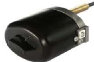
160506 Wiper Motor 12 V., Wiper angle 110°, Wiper shaft w/ 1 Shaft Moment: 0.8NM
