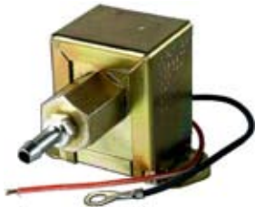
070056 Fuel Pump Servicing: Caterpillar, IH/Case. 24 V., Capacity 113.5 L/h, Pressure (Kg) 0.3 - 0.45, Pressure (Psi) 4.5 - 6
