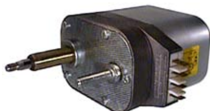
160293 Wiper Motor 24 V., Distance between shafts 57 mm, Wiper angle 110°, Wiper shaft w/ 2 shafts for parallelogram
