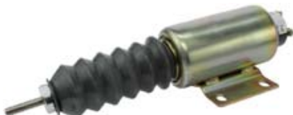
090431 Shutdown Solenoid Servicing: Universal. 24 V., 24 Timermodul V. , 30 Amp. pull , 0.57 Amp. hold , Thread 5/16 - 24, Return spring 17.6 - 26 lbs, Pull rating 165N, Hold rating 391N Syncro start / Woodward.
