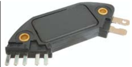
150061 Ignition Module Servicing: AMC, GM, Opel, Vauxhall., Fiat Type Pick up, Terminals 8
