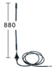
040182 Aerial Colour Black, Length 880 mm, Hole size 18 mm, Mounting angle 0 - 45°, Cable length 1.6 m, Material Fiber glass Removable mast.
