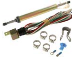
081177 Fuel Heater 24 V., 250 Watt, Type Electric, Demister tube connection 8/10 mm, Sandwich tipe Yes
