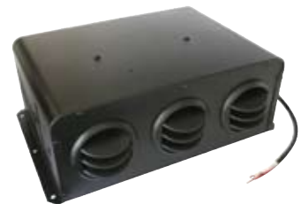
060235 Cabin Heater 24 V., Airflow-Speed 1 264 m³/h, Water connection 16 mm, Regulation Yes
