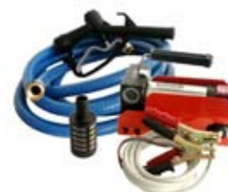
070175 Diesel Transfer/Filter Kit 24 V., Capacity 40 L/min, Type Fluid, Pressure (bar) 1.1 Tank kit 24V 2.5 m suction hose w/ filter. 2.5 m pressure hose w/ pistol. 2 m cord w/ alligator clips, switch on the pump, bypass valve on the pump ensure against overloading. Not gasoline!
