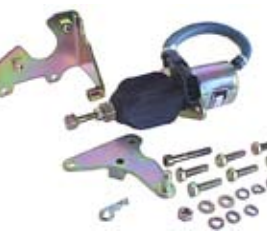
090107 Solenoid Shutdown Kit 1.1 Amp., Pull rating 89N at 25.4 mm, Hold rating 178N Syncro start / Woodward. External.
