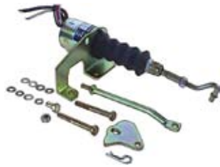
090100 Solenoid Shutdown Kit 0.5 Amp., Pull rating 89N at 25.4 mm, Hold rating 178N Syncro start / Woodward. External.
