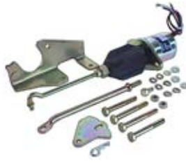
090105 Solenoid Shutdown Kit Servicing: Nippodenso, Zexel. 0.63 Amp., Pull rating 89N at 25.4 mm, Hold rating 178N Syncro start / Woodward. External.
