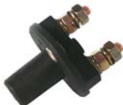
180313 Battery Main Switch 24 V., 500 Amp. (5 min), 100 Amp.-Cont, Type Battery, No. of mounting holes 2, Mounting holes distance 45 mm, Key No, Protection degree IP 4x Spare key: Cargo 180029 or 180143. Rubber protection cap: Cargo 180374.
