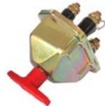
180276 Battery Main Switch 24 V., 2500 Amp. (5 min), 250 Amp.-Cont, Type Battery, No. of mounting holes 2, Mounting holes distance 110 mm, Material Plastic, Poles 2, Key Yes, Waterproof Yes, Explosionproof Yes, Protection degree IP 667 Rubber boot: Cargo 180375. For alternator w/ integral regulator. W/D+ contact.
