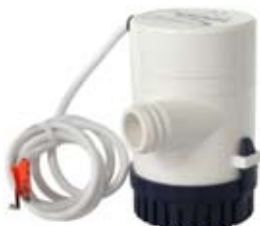
070155 Bilge Pump 12 V., Capacity 63 L/min, Type Bilge, Lift height 4 m, Dimension 124.7 x 78, Hose connection 28.6 mm Model UP1000.
